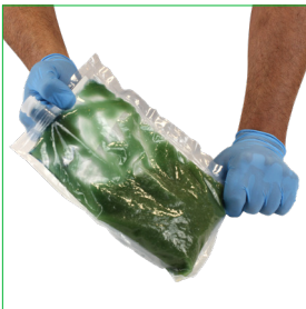
Visible colour change. Mixture is ready to pour.
