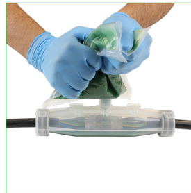
Place the spout on the mould body, quarter turn to release the resin and fill the kit.
