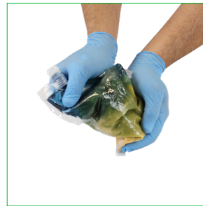
2 minutes: Resin turns green, indicating perfect mix
