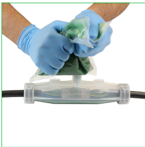
Place the spout on the mould body, quarter turn to release the resin and fill the kit.
